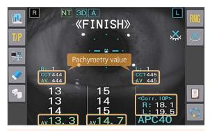
The pachymetry data can be used to display a corrected IOP value.
