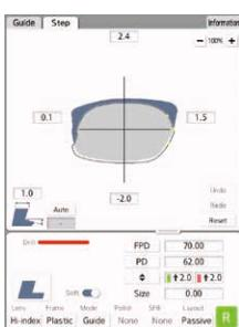
To further enhance precision, the ME-1 features variable step angle control, which maintains a uniform step width across the entire lens shape. This prevents the base of the step from becoming thinner, which leads to a consistent accurate fit, even in complex frame geometries, delivering professional-grade results with every lens.
